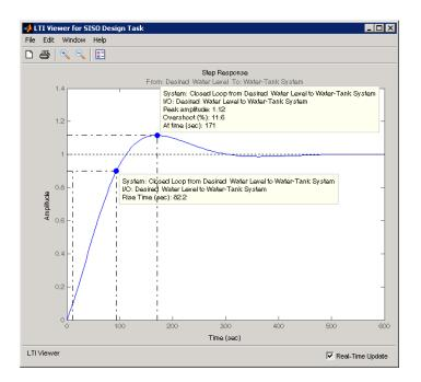
This system response with the PID compensator exceeds the maximum allowed overshoot of 5%. The rise time is much slower than the required rise time of 5 seconds.
