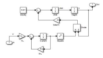
The Magnetic Ball Plant model represents an iron ball of mass M. This ball moves under the influence of the gravitational force, Mg, and an induced magnetic force,  $\frac{\beta i^2}{h}$ . The presence of the squared term in the induced magnetic force results in a nonlinear plant.
