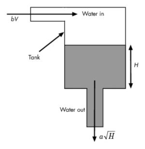
Water enters the tank from the top at a rate proportional to the voltage, V, applied to the pump. The water leaves through an opening in the tank base at a rate that is proportional to the square root of the water height, H, in the tank. The presence of the square root in the water flow rate results in a nonlinear plant.
