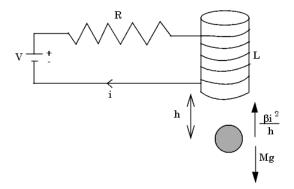
The following table describes the variables, parameters, differential equations, states, inputs, and outputs of the Magnetic Ball Plant subsystem.
