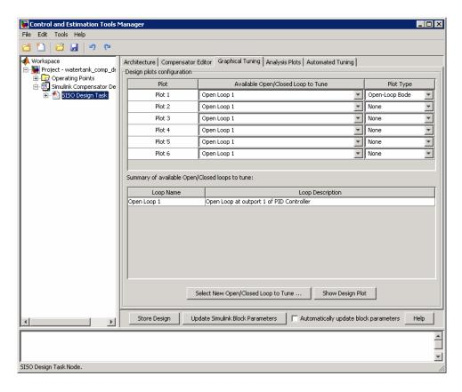
This action creates an Open-Loop Bode plot in the SISO Design for SISO Design Task window. This plot shows a Bode plot of the linearized model with the compensator designed using automated PID tuning.
