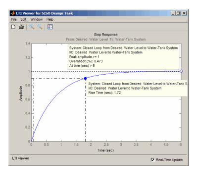
This compensator design satisfies the design requirements of less than 5% overshoot and less than 5 second rise time.
